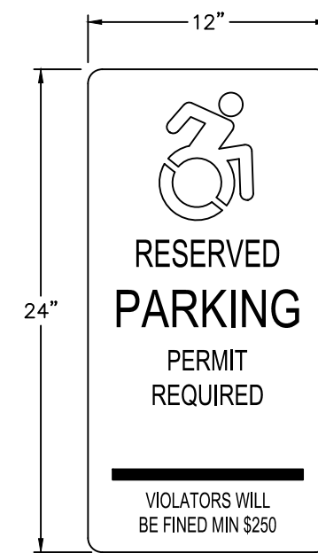
RESERVED PARKING SIGN SCALE: N.T.S. NOTES: CDOT NUMBER: ALUMINUM THICKNESS: .080" BACKGROUND: BLUE (REF.) LEGEND: SILVER (REF.) POSTS: SEE "RESERVED PARKING SIGN AND POST" DETAIL
